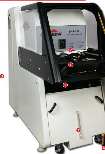
New, easy-to-maintain standard coolant system is almost 60 percent larger than earlier machine models at 208 L (55 gallon) capacity and is equipped with PF filter cartridge, magnetic separator, quick disconnect lines, and a level gage. Large capacity pump delivers double the flow rate. The system removes from the front on easy-to-roll casters.
